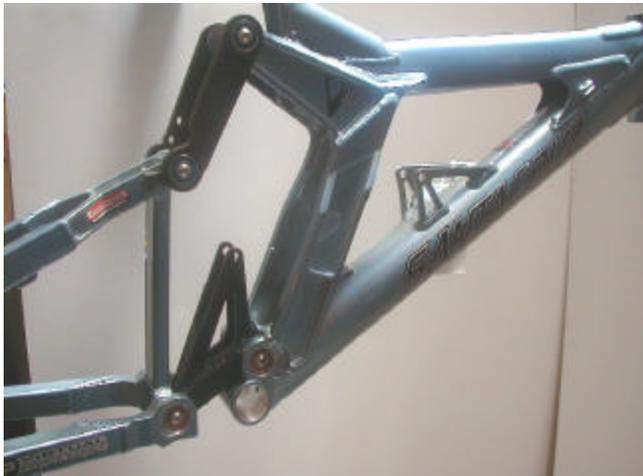
Use a 6mm allen wrench to remove the link stop bolt behind the right side upper link. Preload the shock by pushing up on the swingarm so the link doesn't push the bolt and trash threads as you're unscrewing it.
